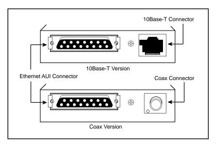
Figure 1-2. GPIB-ENET Side Panel
